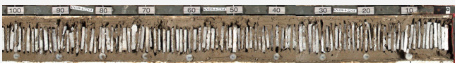
"Curated sediment core from the North Atlantic that has undergone high-resolution sampling (evident from the styrofoam acting as a place-holder/marker for the missing mud). The samples have been used for C-14 dating, isotope studies, foram and IRD counts, and paleomagnetism." Nichole Anest, Interim Curator, LDEO
