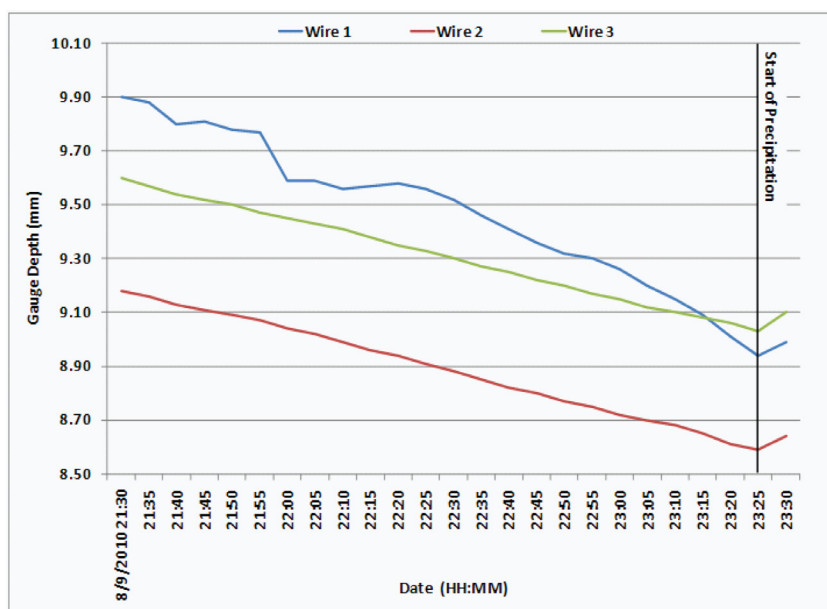
Figure 21. Five-minute gauge depths from wire 1 (blue), wire 2 (red) and wire 3 (green) at Monahan, TX from August 8 th 2010 21:30 UTC to 23:30 UTC. Reported wire depths are purposely offset with relative changes per wire indicating the magnitude of gauge evaporation loss.
