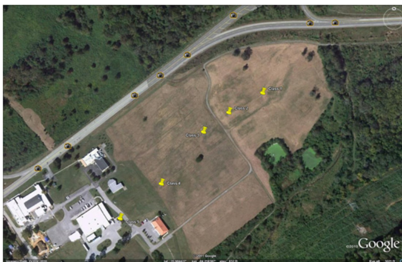
Figure 7. Active temperature controlled steel building and parking area located near Oak Ridge, TN. Five sampling sites (yellow pins) are seen northeast of the thermal source, corresponding to USCRN thermal site score classes 5 (closest) through 1 (furthest).
