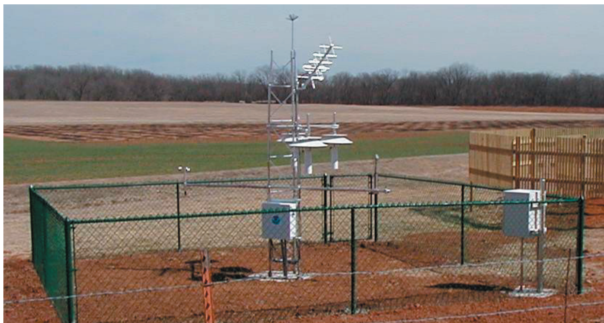
Figure 1: A typical USCRN installation (Stillwater 5 WNW, OK). The meteorological sensors and datalogger are mounted on the 3-meter tower, inside the green-fenced area. Protection is used on the cabling that runs from the datalogger to the cross-members on which the instruments are mounted. (Note: The installation in the photograph is shown before the protection was installed.)
