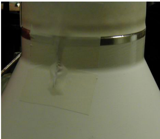
Figure 4: Exterior of the gauge with the waterproof roofing material and white vinyl tape applied.
