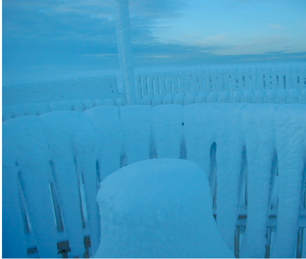
Figure 11: Barrow, AK Geonor inlet (blocked and capped by rime ice) with AC site program.
