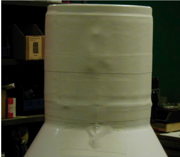
Figure 5: Finished exterior of the gauge with the heater installed and covered.
