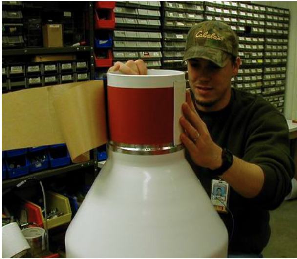
Figure 1: Installing the outside inlet heater strip.
