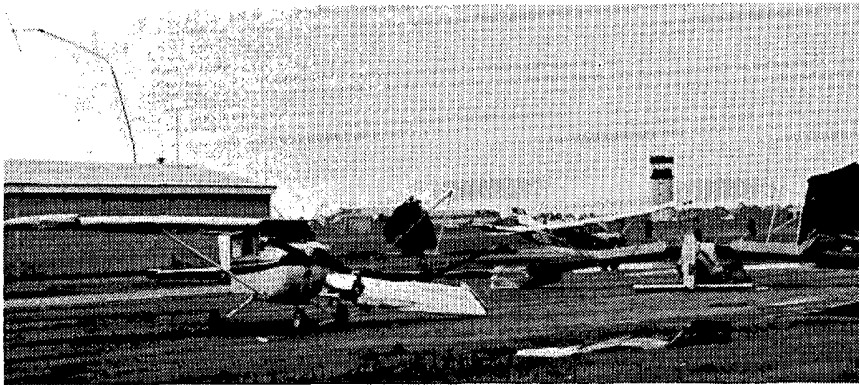
ABOVE: Examples of hangars that collapsed onto aircraft at Hooks. BELOW: Aircraft that were damaged or flipped by diverging winds at Hooks, left, and a plywood missile that was imbedded nearly a foot into the ground at the airport. ---All four photos by Tim Marshall, Haag Engineering Co.
