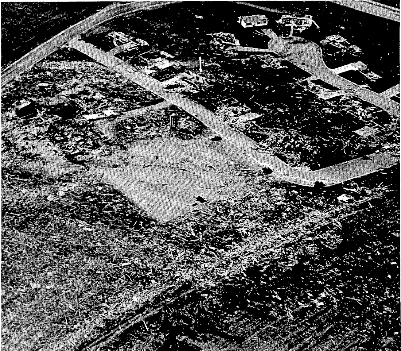
An aerial view of the subdivision which received F5 damage and where 7 deaths occurred. The homes were disintegrated by the tornado and debris was scattered for a considerable distance. The Lutheran Church appears at the left edge of the photo. (CT)
