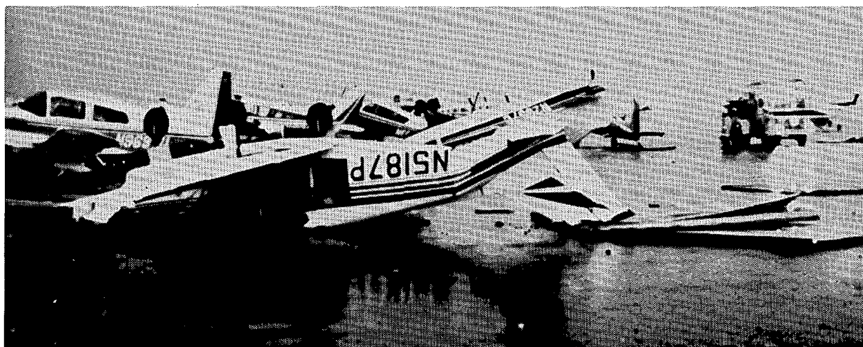
A panoramic view from southeast (left) to west (right) of the damage at JEFFCO. Made from 5 individual pictures, this scene shows large panels of sheet metal which were torn from hangars and scattered by the microburst winds. A plane which was flipped over (shown at center) is enlarged below.
