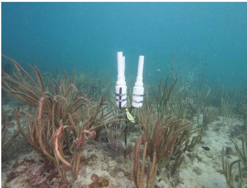
Figure 3. Sediment traps installed at all offshore sites for environmental monitoring of hardbottom and reef resources in Cuts 1 and 2.
