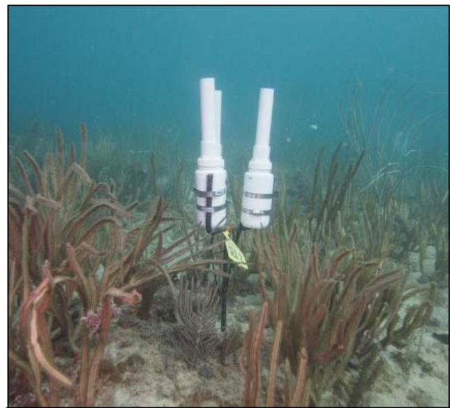
Figure 3: Sediment traps installed at all offshore sites for environmental monitoring of hardbottom and reef resources in Cuts 1 and 2.
