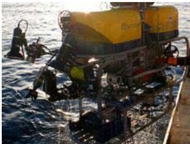
Figure 2. Kraken 2 ROV, 1000-m working depth, equipped with HD camera, still camera, manipulator arm. Sampling array is mounted on sled beneath vehicle.
