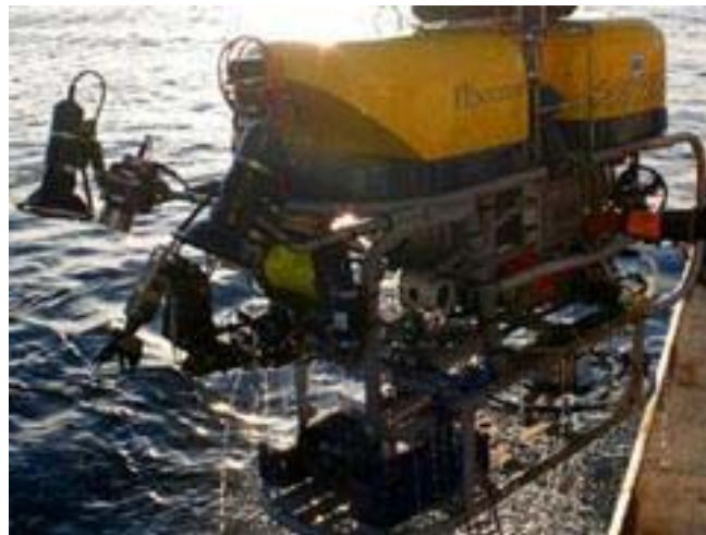
Figure 3. Kraken 2 ROV, 1000-m working depth, equipped with HD camera, still camera, manipulator arm. Sampling array is mounted on sled beneath vehicle.
