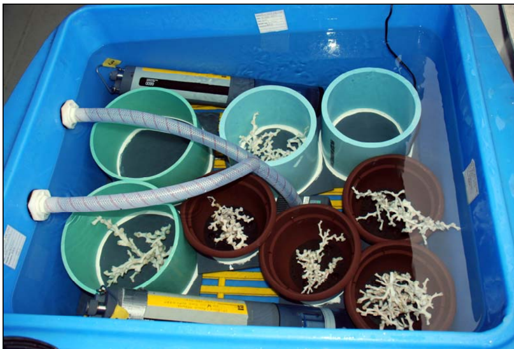
Figure 8. Insulated holding tank used to keep coral colonies alive at 7-8° C. Portable chiller not shown. Two YSI data loggers used for coral respiration experiments appear at top and bottom of photo. Tank is normally covered.
