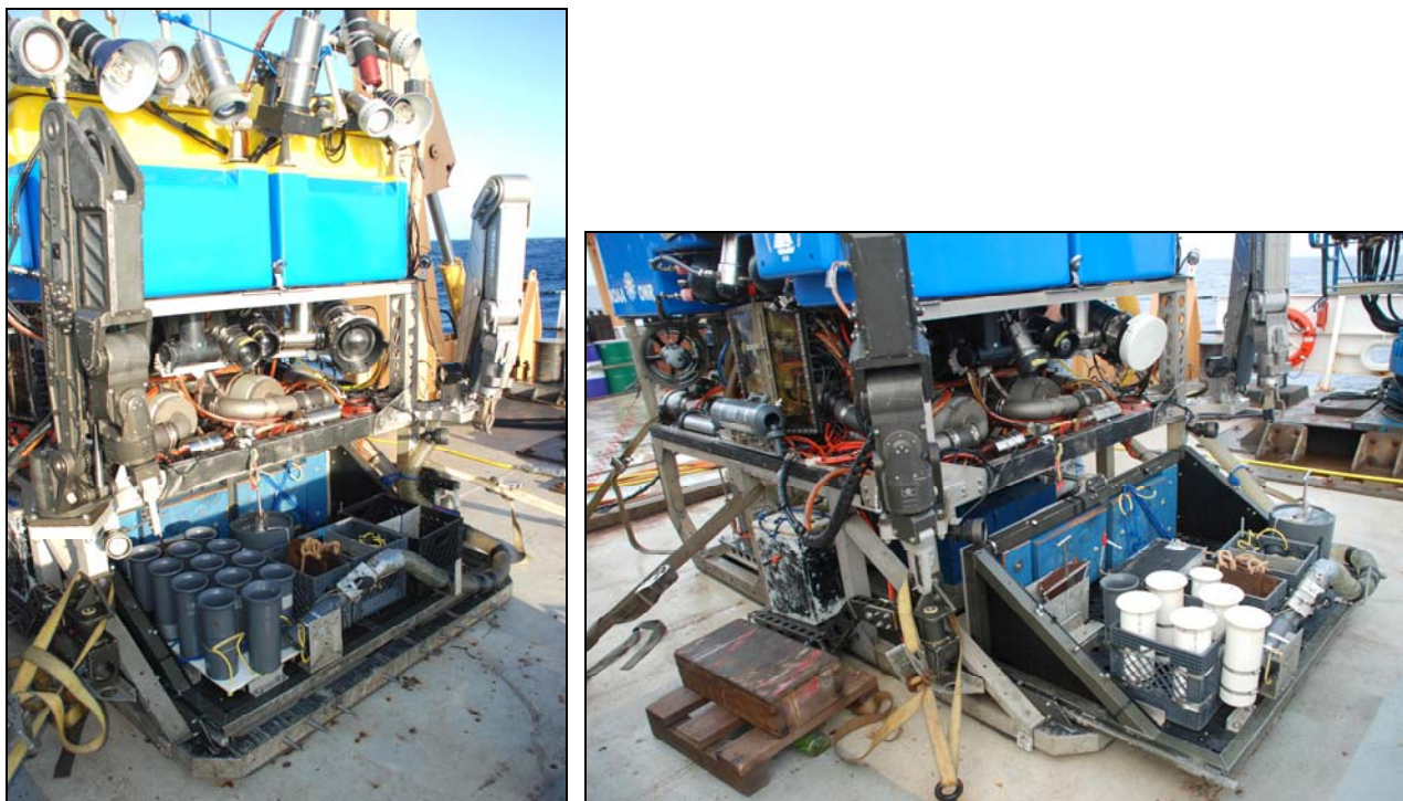
Figure 4. Front views of Jason II ROV illustrating extended front work tray with 12 PVC quivers used for most dives. After this rack was lost, it was replaced by the quiver arrangement in right panel. Round biobox with T-handle can be seen in both photos as can other milk crates and a rectangular sample box (right). HD video science camera with adjacent mounted still camera is visible to port side of vehicle, uncovered (left) and covered (right).
