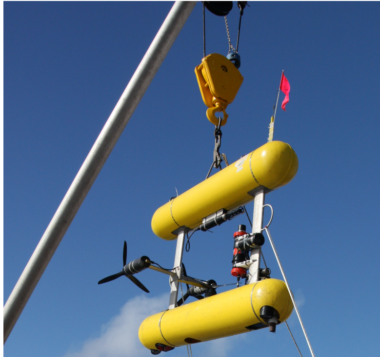
Figure 3. SeaBed type Autonomous Underwater Vehicle, Lucille , being deployed from research vessel.
