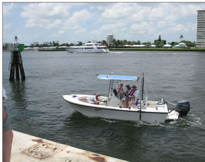
Figure 7. Vessel equipped with down-looking, 1200-kHz ADCP used to survey the Port Everglades Channel bathymetry and collect calibration velocity data.
