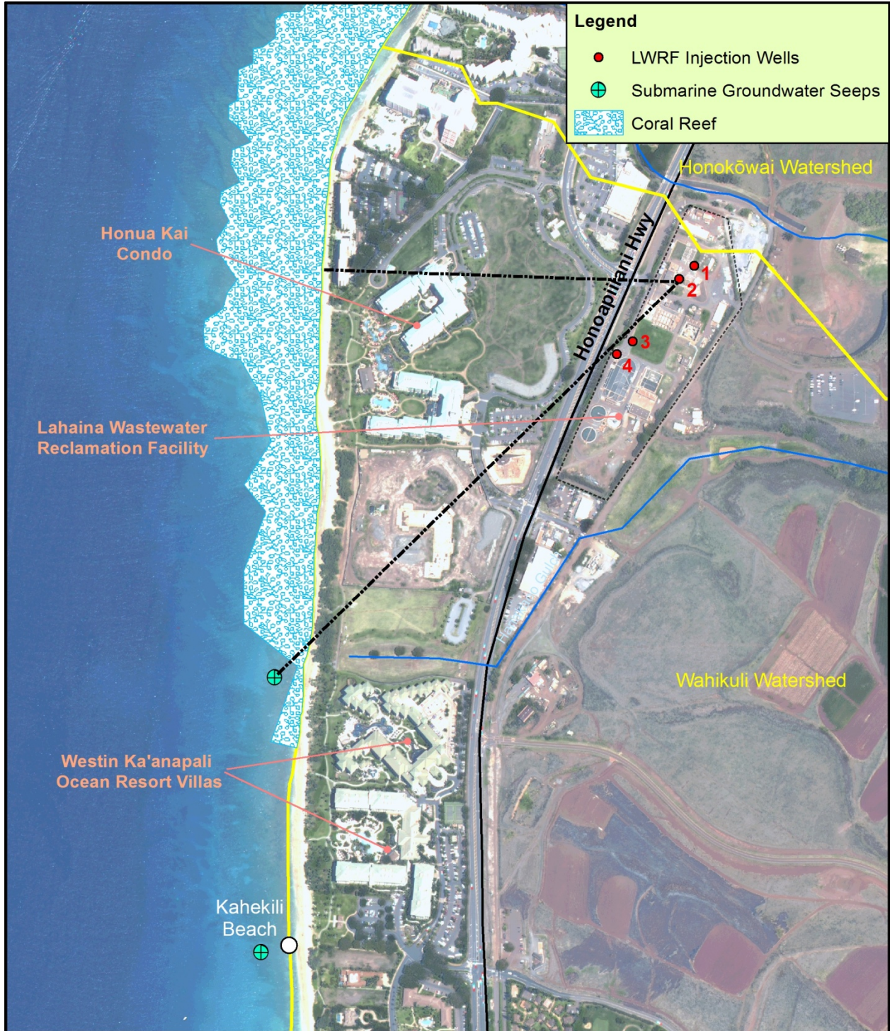
Figure 31. Lahaina WWRF and Submarine Ground Water Seeps
