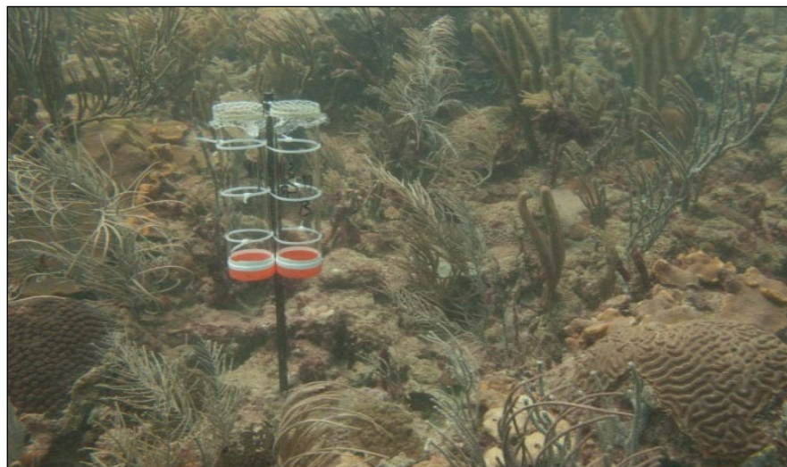
Figure 4.2. Simple tube traps used to collect suspended sediments. Sediment traps were clear plastic tubes 30-cm high with an internal diameter of 6.4 cm. Tops of the traps were covered with a 1 cm 2 nylon mesh to prevent entry of small fish and invertebrates. Traps were secured with plastic cable ties to steel rods that were driven into the hard reef surface. Traps were situated so that the tops of the traps were ~60 cm above the surrounding seafloor.
