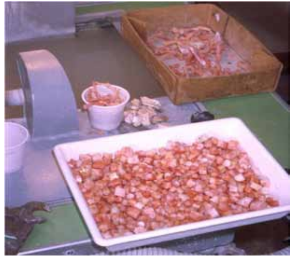
Fig. 2. Corallium elatius branches cut into smaller, uniform shapes called bead blanks. Torre del Greco, May 2000, S.J. Torntore.
