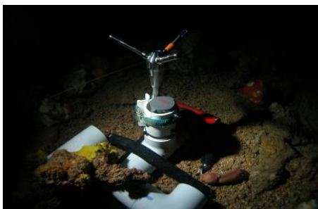
Figure 3: Nortek Vector Velocimeter mounted on a PVC deployment pod and weighted in place
