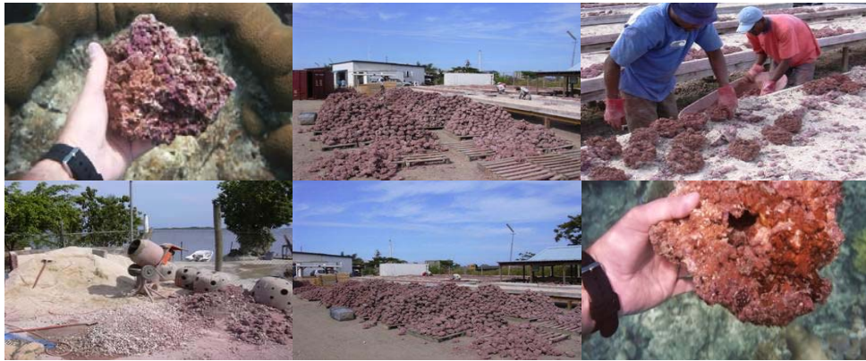
WSI cultured live rock production at Lautoka. Iron oxide pigment imparts pink-purple colour further developed by coralline algae during seasoning on the reef
