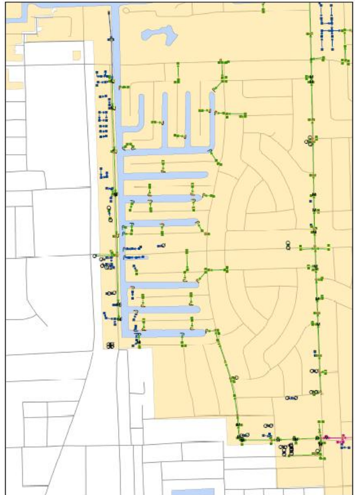
Figure 9. The detailed storm drain network data available in the City of Fort Lauderdale is a powerful resource for the watershed manager, but ends at the city line (unshaded area).
