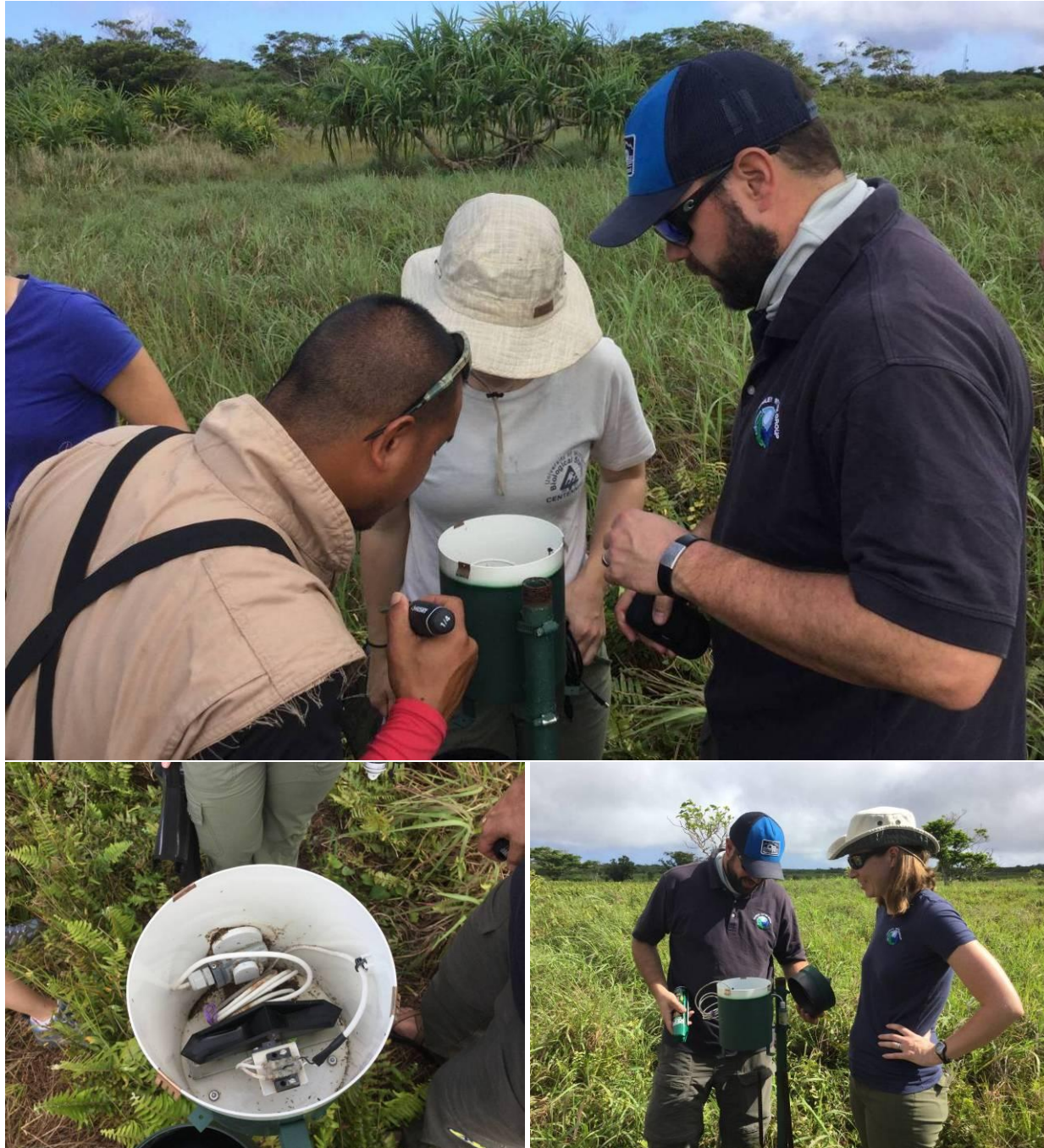
Figure 16. Rain gauge on the Sabana Plateau-TKRG4(top); ant nest affecting the tipping bucket (bottom left); removing ants from rain gauge (bottom right).
