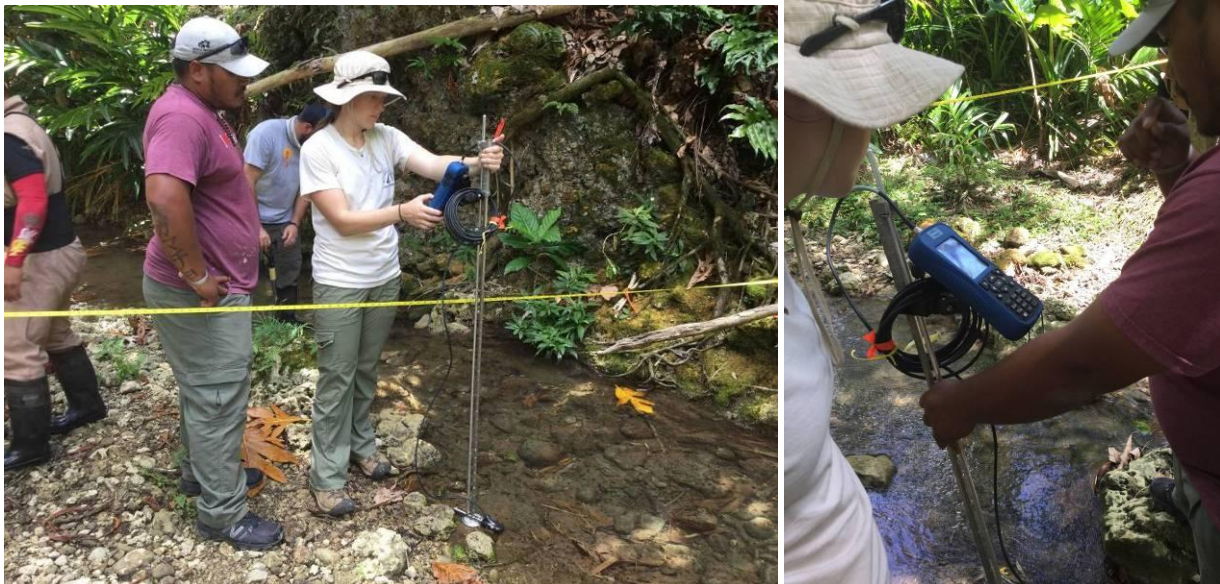
Figure 22. Using the HACH portable flow meter in the field.
