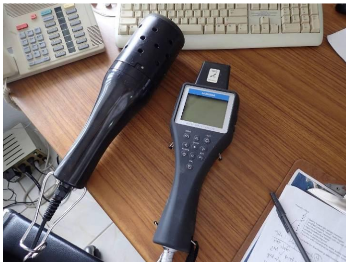
Figure 21. HORIBA multiple parameter meter used in Phase I (left); YSI 556 MPS meter used in Phase II (right)
