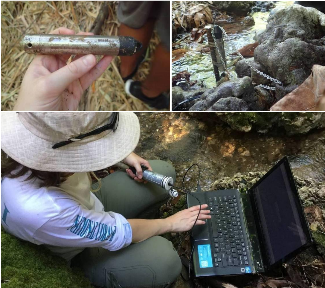
Figure 18. HOBO level loggers were used for determine barometric pressure ("air" loggers; left photo); stream depth (attached to rebar in stream; right photo); and downloading logger data onto laptop in the field (bottom).
