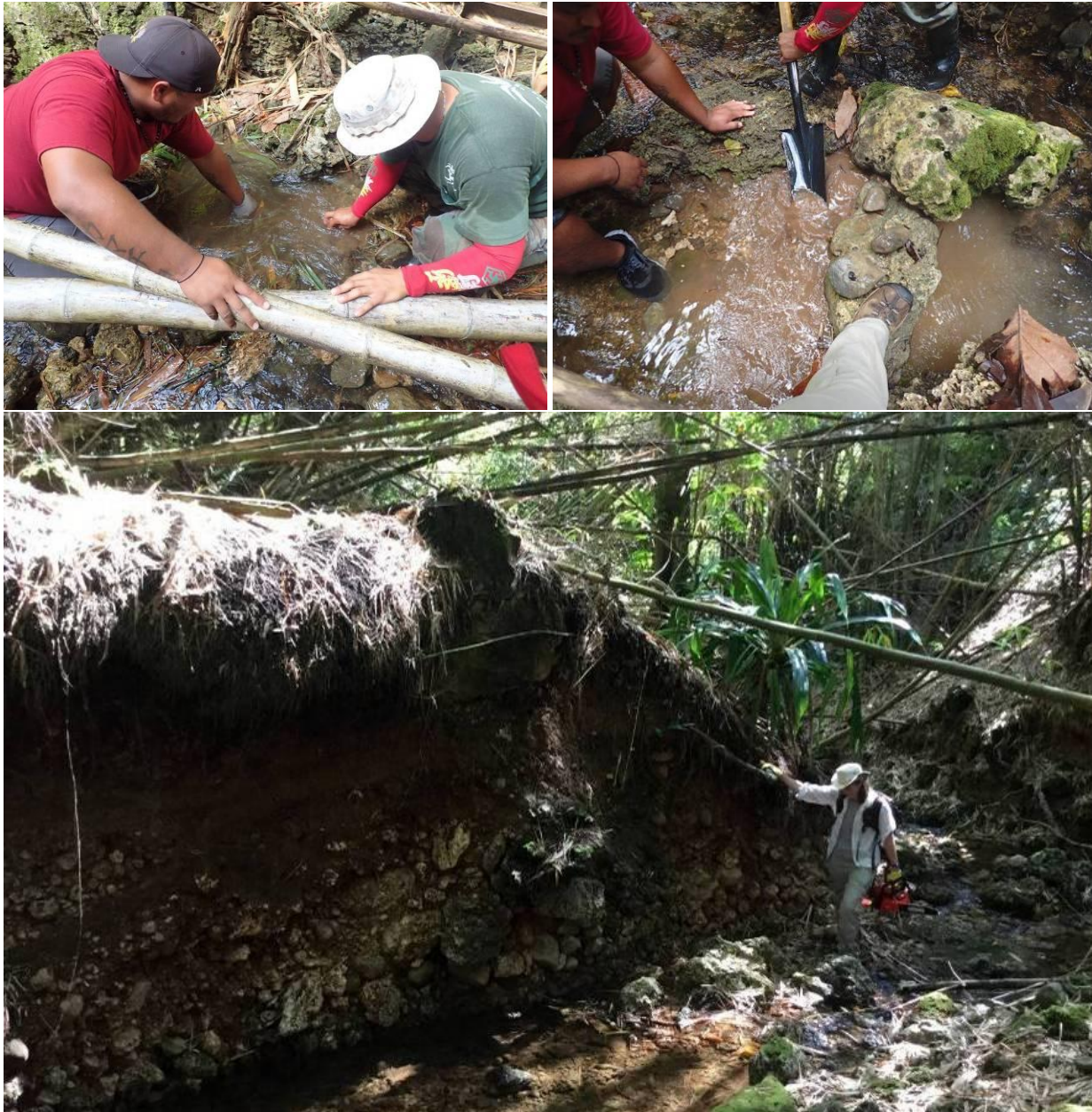
Figure 9. Field team searching for logger under bamboo at TK1-R2 (left); removing sediment build-up at Station TK1-R3; and carrying in a chainsaw to improve access and break-up a debris dam at TK1-R1 (bottom).
