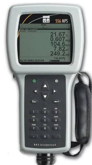
Figure 21. HORIBA multiple parameter meter used in Phase I (left); YSI 556 MPS meter used in Phase II (right)
