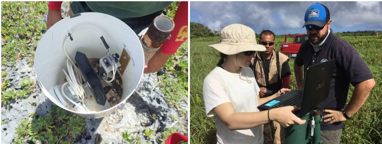
Figure 17. Inside of rain gauge showing tipping bucket (bottom left); Downloading data from the Hoboware Rain Gauge (right).
