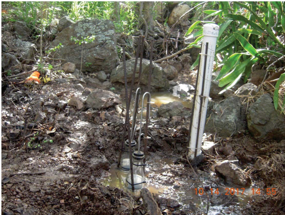
Figure 24: A peak crest gauge and single stage samplers in Punta Aloe North Stream
