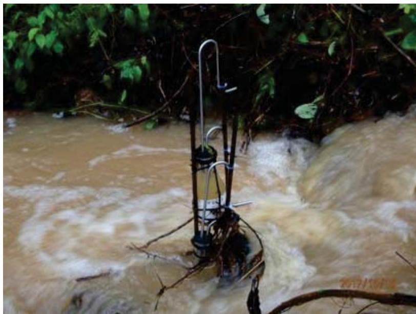
Figure 26: Single Stage Samplers in Punta Aloe North Stream during 15 October 2017 storm
