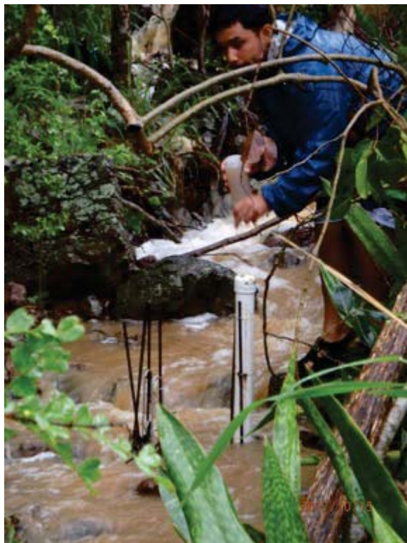
Figure 25: Grab sample collection in Punta Aloe North Stream during 15 October 2017 storm
