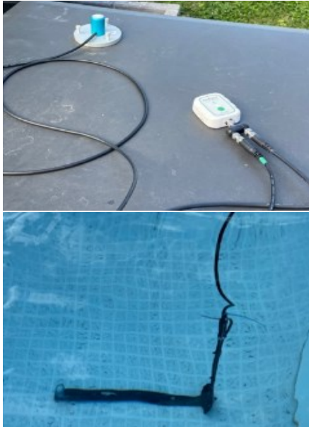
Figure 4. APOGEE Photosynthetic Active Radiation (PAR) above-water (upper panel) and below-water (lower panel) sensors.
