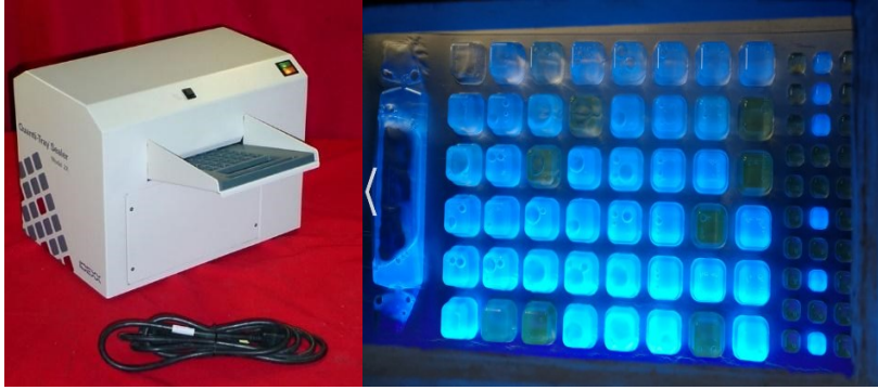
Figure 6. Illustration of the IDEXX Quanti-Tray system: Sealer (left panel) and Quanti-Tray Legiolert (right panel).
