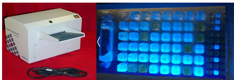
Figure 10. Illustration of the IDEXX Quanti-Tray system: Sealer (left panel) and Quanti-Tray Legiolert (right panel).
